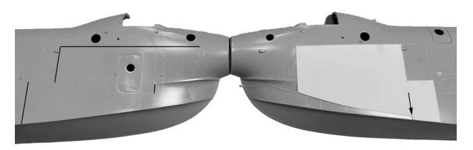
Aft Fuselage/Hull Modification: Using the raised panel lines (Highlighted in BLACK) on aft Fuselage/Hull as a reference, use a straight edge and knife or scriber to cut away the kit Vertical Stabilizer. Cut at the panel line where the Vertical Stabilizer meets the Fuselage/Hull.
